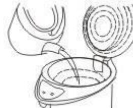
Press the lid opening switch to unlock the lid's top cover and open it.
